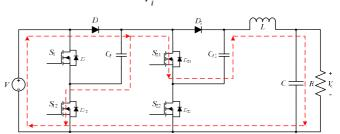
Figure 2. Power flow of the 2-plus-D converter in mode 1.
