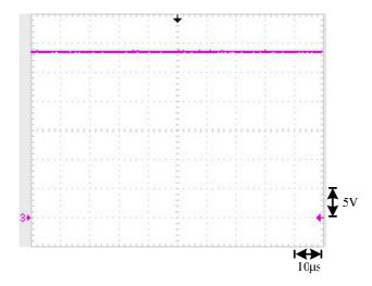
Figure 12. The steady-state output voltage 28V.
