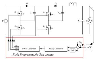
Figure 10. Block diagram of the overall system.
