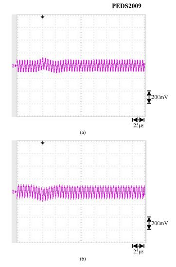
Figure 13. Measured load transient response due to load change for the 2plus-D converter. (a) From rated load to no load. (b) From no load to rated load.
